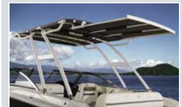
A permanent rigid structure with a stretched canvas top covering, and the extendable sunshade aft. Available for models 23SC and 25SC.
